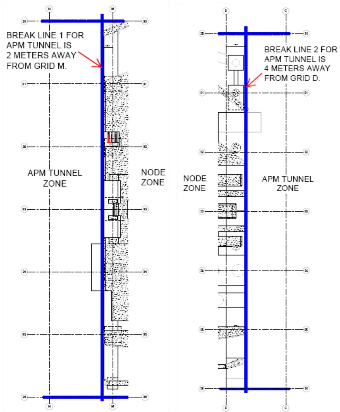
Figure 5 BIM Model Zone Break Line at Node / APM
