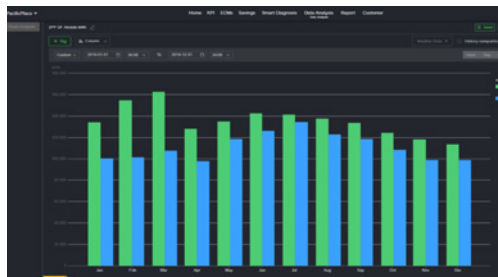
Airside Electricity Consumption Comparison of Before and After Installation of EC Plug Fan
