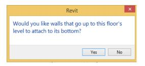
If "Yes" is selected, the volume of the structural walls below will be measured to the underside of the slab, as shown for the wall on the left below.
