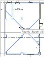
By defining the floor level above a room as the Upper Limit, and entering the slab thickness in negative value as the Limit Offset, the reported Unbounded Height will give the floor to ceiling soffit height, which should be good for generating the wall and column surface areas. Adjustment would need to be made for the beam surfaces and end junctions. Adjustment for window and door openings may be taken care of when processing the window and door quantities.
